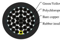
Green/Yellow wire Polychloroprene rubber outer jacket Bare copper conductor Rubber insulation
